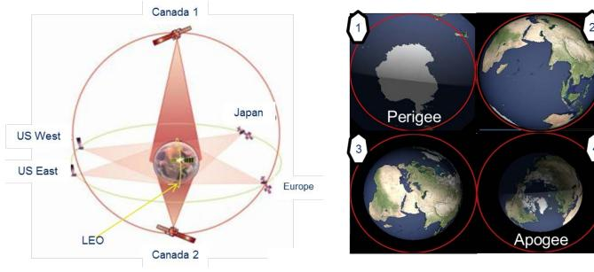
Figure 4: Two satellites provide continuous coverage
