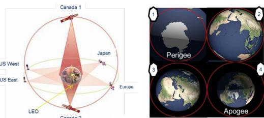
Figure 4: Two satellites provide continuous coverage
