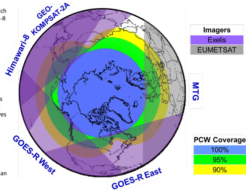
Figure 1: ABI on PCW fills geostationary imager constellation Arctic gap
